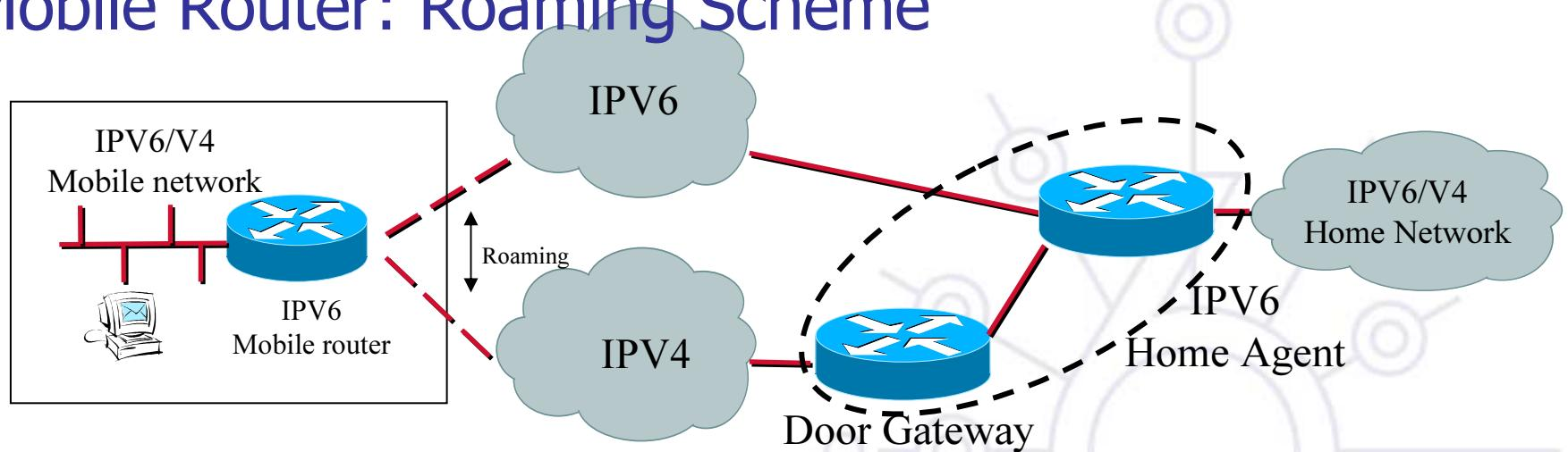
Mobile IPv6 router roaming into a V4 or V6 network
